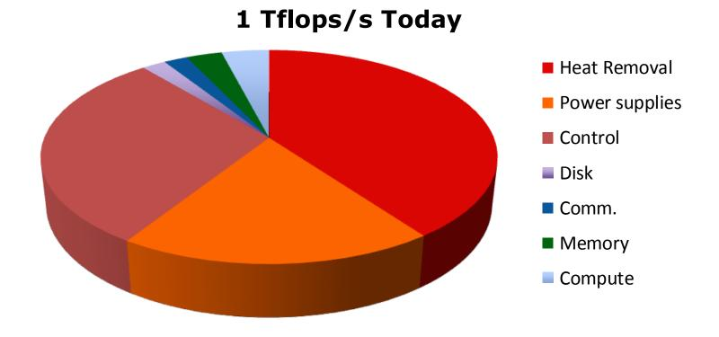
A SIMD accelerator approach gives up Control to reduce wattage per TFLOPS. Which can work, for some applications that are very regular and SIMD-like: vectorizable with long vectors
